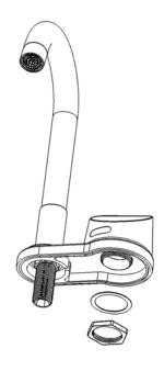
4. Install the washer and nut to secure the control panel to the deck plate
