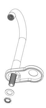
2. Install the washer and nut to secure the faucet to the deck plate
