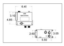
The automatic smart water flush mode is activated when the faucet has been idle for a pre-determined amount of time. The default setting is full cold water flow for 10 seconds after six hours of faucet idle time. The Muirsis MCPF series faucets utilize a total hands-free method. They are specifically designed for the healthcare industry. All the functions are controlled with the control panel and indicated with LED's. All functions are achieved by a single hand movement.
