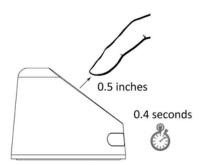
For the sensors to operate properly, your finger must be held right below the LED, at a height of 0.5 inches. Your finger must be held steadily for a duration of 0.4 seconds.
